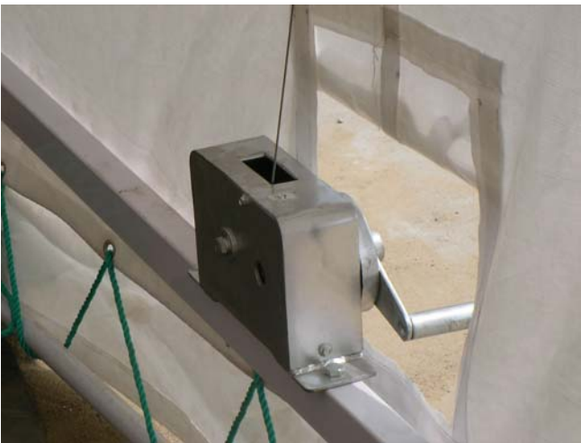
Winch Assembly Mounted To Lower End panel Beam
